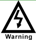
WARNING: ENSURE THAT POWER IS DISCONNECTED FROM THE VENDER OR THAT THE POWER INTERRUPT SWITCH IS NOT DEFEATED BEFORE INSPECTING OR REPLACING THE LAMPS, OTHER ELECTRICAL COMPONENTS, OR WORKING WITH OR ADJUSTING THE VENDING MECHANISM. FAILURE TO COMPLY WITH THESE INSTRUCTIONS MAY SUBJECT THE USER TO THE RISK OF ELECTRICAL SHOCK OR MECHANICAL INJURY, WHICH CAN BE SERIOUS OR FATAL.
